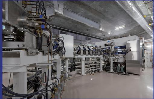
30 MeV Cyclotron and Beam Transport System
