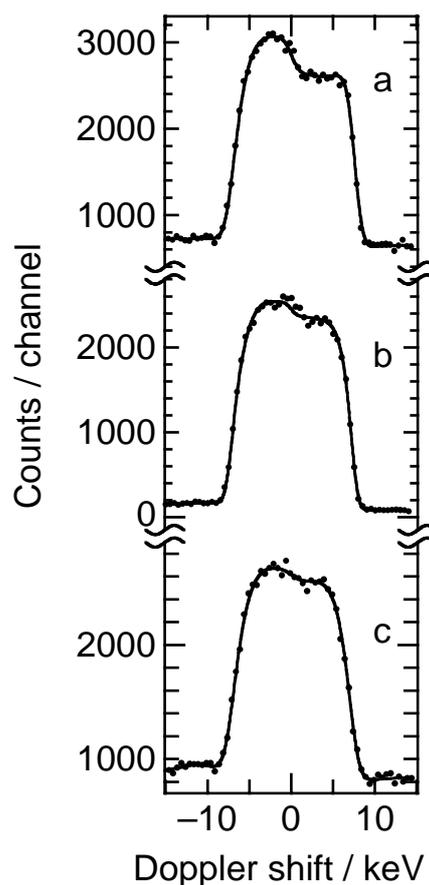
**Figure 3.** Spectral lineshapes of prompt  $\gamma$ -ray of 478 keV of  ${}^7\text{Li}$  measured for air/B/Si (a), methanol/B/Si (b), and glycerin/B/Si (c). The abscissa indicates the Doppler shift from 478 keV.
