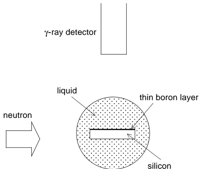
**Figure 1.** Conceptual arrangement for the measurement using a B/Si wafer. The thickness of boron layer was 50 nm and the wafer size is  $1 \times 1$  cm<sup>2</sup>. The distance between the wafer and the detector was 30 cm. The B/Si wafer was immersed in a liquid sample and the boron layer was set perpendicular to the measurement axis.
