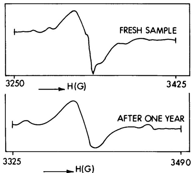
**Figure 3.** EPR spectra of  $^{239}\text{Pu(IV)}$ -doped PVA film, stored for different times.
