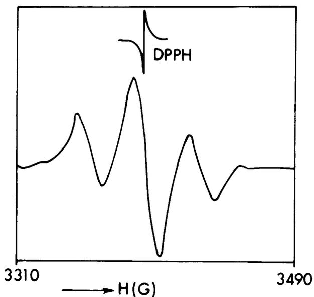
**Figure 1.** EPR spectrum of gamma irradiated (dose 4 kGy) PVA film at room temperature.
