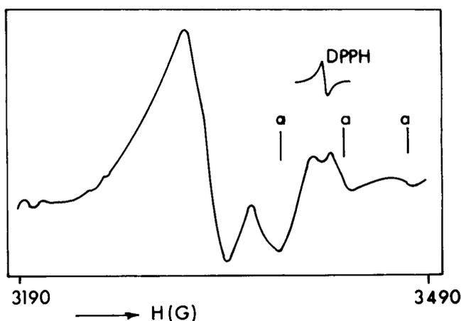
**Figure 2.** EPR spectrum of gamma irradiated (dose 4 kGy) U(VI)-doped PVA film. The weak triplet marked by 'a' at  $g = 2.001 \pm 0.001$ .
