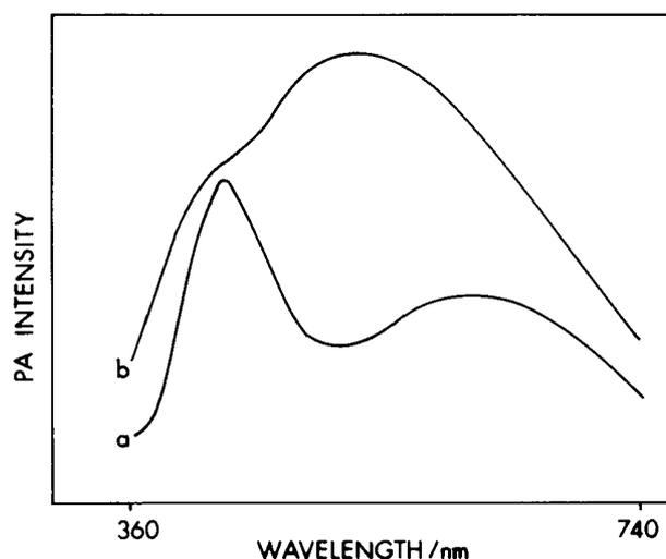
**Figure 4.** PA spectra of U(VI)-doped PVA film (a) nonirradiated (b) gamma irradiated at 4 kGy.
