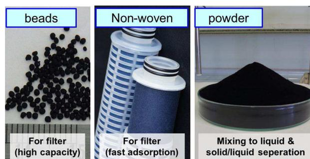
Fig. 2. Various Cs-adsorbents with Prussian blue nanoparticles
