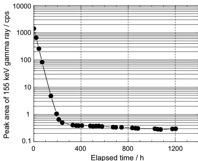
Figure 3. Determination of  $^{188}\text{W}$  breakthrough in the  $^{188}\text{Re}$  effluent.
