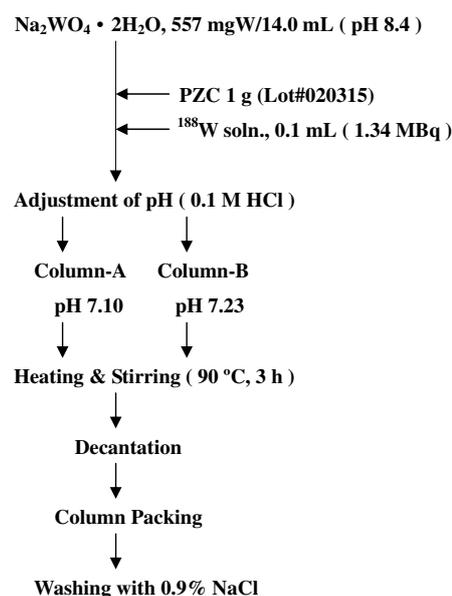
Scheme 1. Preparation of  $^{188}\text{W}/^{188}\text{Re}$  generators based on PZC.
