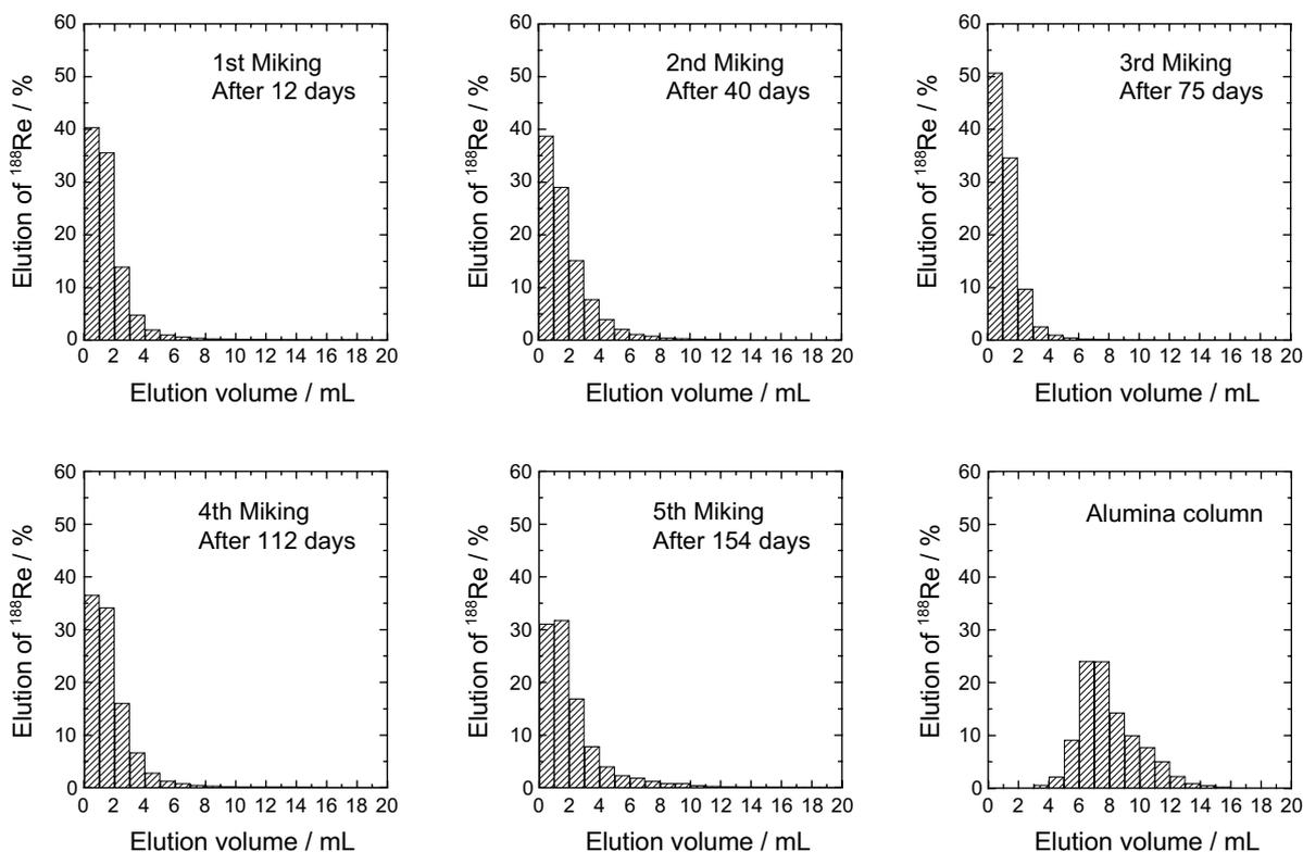
Figure 1. Elution behavior of  $^{188}\text{Re}$  from the PZC generator (PZC column: 8 mm $\phi$   $\times$  32 mm, alumina column: 10 mm $\phi$   $\times$  60 mm).
