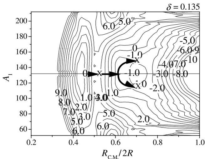
**Figure 10.** The contour plot of the PES in the case of  $\delta = 0.135$  for  $^{264}\text{Fm}$ . The abscissa denotes the distance between the centers of mass of future fission fragments and the ordinate the mass number of a fission fragment. The solid line shows the mass-symmetric division.  $R$  is the radius of the fissioning nucleus. Arrows show expected fission paths.
