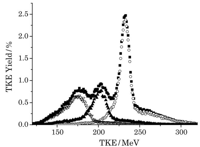
**Figure 7.** Decomposition of the TKE distribution according to the three components of the deformation parameter  $\delta$ . Open circles denote Component I, solid upward triangles Component II, and open downward triangles Component III. Solid squares denote the sum of the three components.
