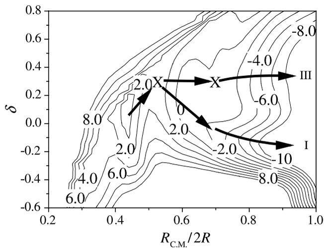
**Figure 9.** The contour plot of the PES for the mass-symmetric fission of  $^{264}\text{Fm}$ . The abscissa denotes the distance between the centers of mass of future fission fragments and the ordinate the deformation parameter  $\delta$ .  $R$  is the radius of the parent nucleus. The first and the second saddle points are marked by X's. Arrows show expected fission paths.
