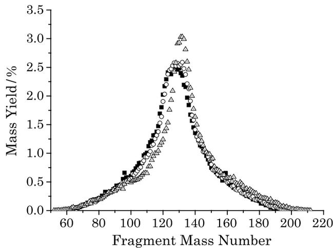
**Figure 12.** Isotope dependence of the mass distribution for the fission of  $^{256,258,264}\text{Fm}$  at the excitation energy  $E_x = 10.0$  MeV. The solid squares denote the mass distribution of the fission fragments of  $^{256}\text{Fm}$ , open circles that of  $^{258}\text{Fm}$ , and open triangles that of  $^{264}\text{Fm}$ .
