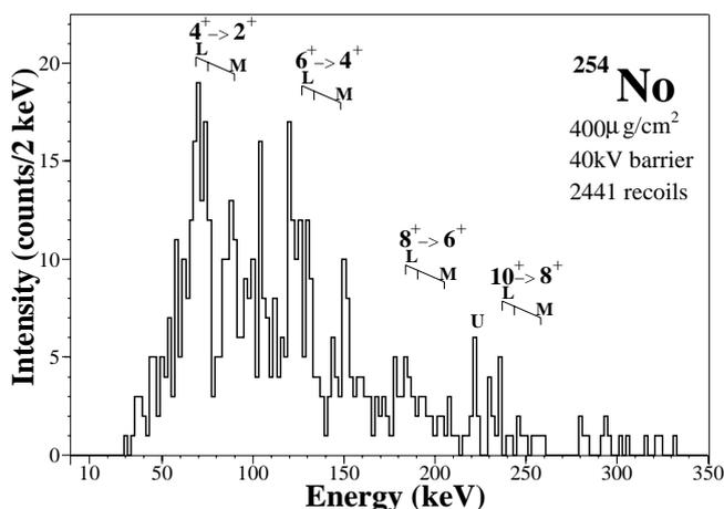
**Figure 2.** Recoil-gated singles conversion electron spectrum of  $^{254}\text{No}$  produced in the reaction  $^{48}\text{Ca} + ^{208}\text{Pb}$  and measured using RITU in conjunction with the SACRED spectrometer.<sup>31</sup>
