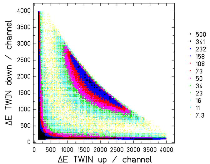
**Figure 4.** Cluster plot of fission fragments recorded by the double ionization chamber in the reaction  $^{238}\text{U} + (\text{CH}_2)_n$ .
