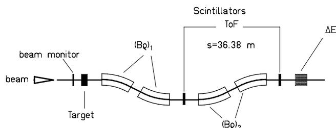
Figure 1. Schematic presentation of the fragment separator and the main detectors.
