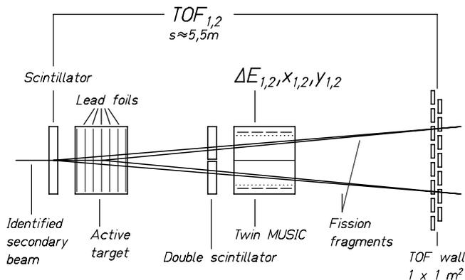
**Figure 3.** Experimental setup to simultaneously measure both fission fragments produced in inverse kinematics (from Reference 7).
