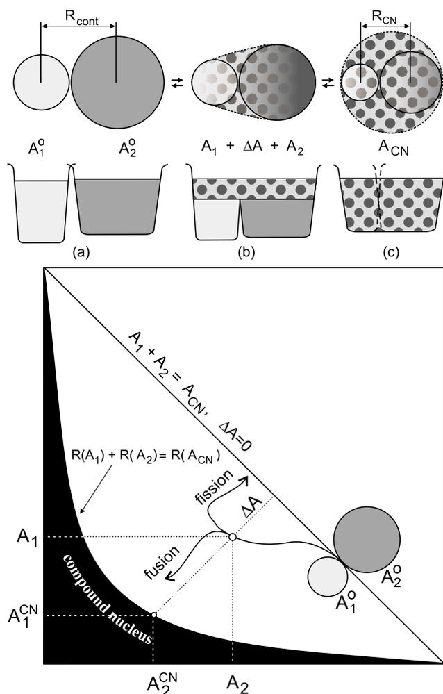
**Figure 1.** Schematic view of the process of compound nucleus formation, fission and quasi-fission in the space of  $A_1$ ,  $A_2$ , and  $\Delta A$ , i.e., the number of nucleons in the projectile-like nucleus, target-like nucleus, and shared nucleons, here  $A_1 + A_2 + \Delta A = A_{\text{CN}}$ .
