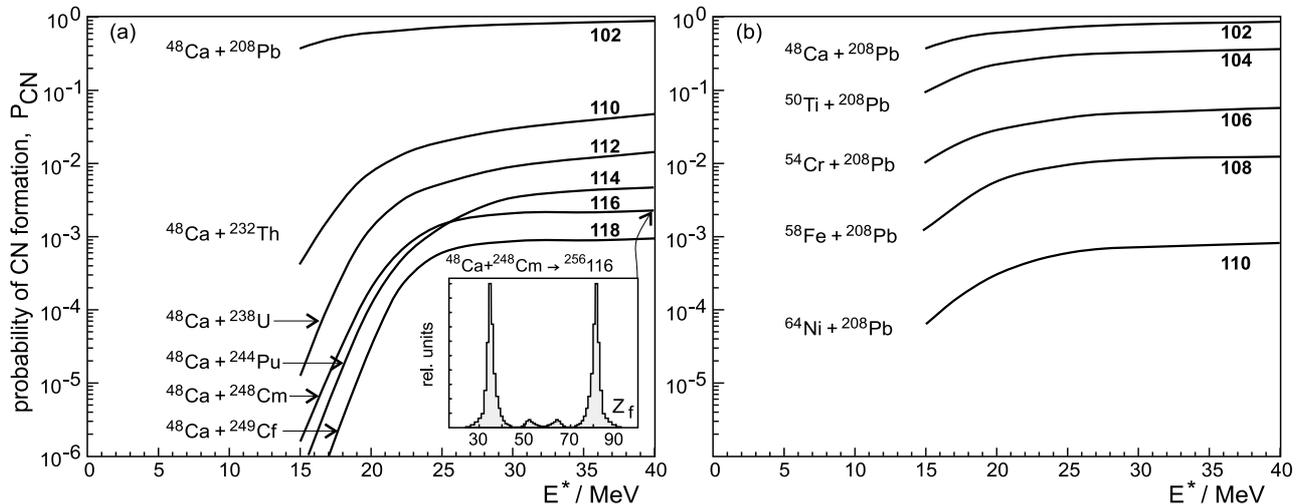
**Figure 4.** Probability of the compound nucleus formation for the (a) “hot” and (b) “cold” fusion reactions. In the inset the charge distribution of quasi-fission fragments is shown for the  $^{48}\text{Ca} + ^{248}\text{Cm}$  fusion reaction at  $E^* = 40$  MeV (linear scale, relative units). The main peaks correspond to the way 1 in Figure 3, whereas the small near-symmetric peaks correspond to the way 2.
