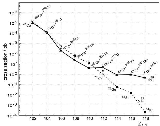
**Figure 5.** Cross sections for formation of heavy evaporation residues in “hot” (triangles,  $3n$  evaporation channel) and “cold” (squares,  $1n$  evaporation channel) fusion reactions. The open symbols correspond to the experimental values, whereas the solid ones to the calculated cross sections. For the “hot” fusion reactions the corresponding projectile-target combinations are shown. For the “cold” fusion reactions  $^{208}\text{Pb}$  is used as a target and only the projectiles are shown.
