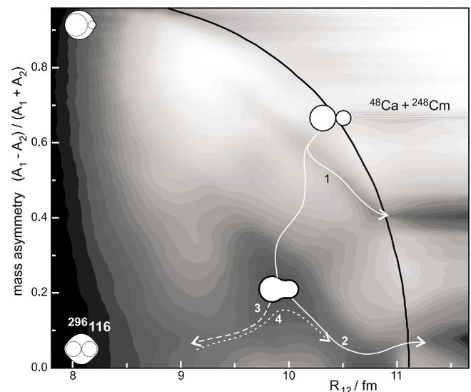
**Figure 3.** Driving potential  $V_{fus-fis}$  as a function of mass asymmetry and distance between centers of two nuclei with zero deformations. The black solid curve corresponds to the contact configurations. The ways 1 and 2 lead to the asymmetric and near-symmetric quasi-fission channels, whereas 3 and 4 correspond to the compound nucleus formation and its regular fission, respectively. See a conformity with Figure 2.
