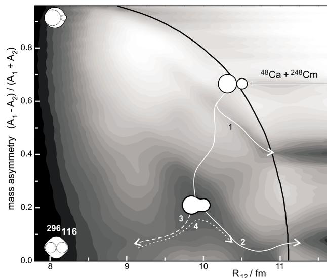
**Figure 3.** Driving potential  $V_{fus-fis}$  as a function of mass asymmetry and distance between centers of two nuclei with zero deformations. The black solid curve corresponds to the contact configurations. The ways 1 and 2 lead to the asymmetric and near-symmetric quasi-fission channels, whereas 3 and 4 correspond to the compound nucleus formation and its regular fission, respectively. See a conformity with Figure 2.
