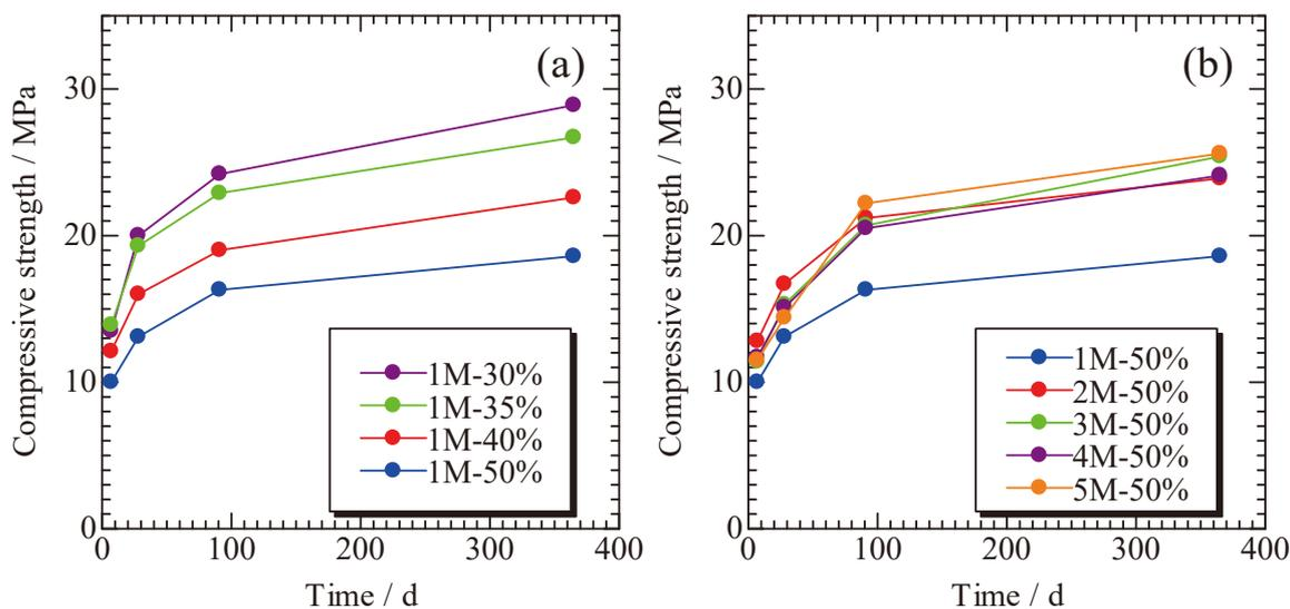
**Figure 2.** Temporal changes of the compressive strengths for samples prepared using various amount of 1 M NaOH solution (a) and using constant amount of 1–5 M NaOH solution (b).
