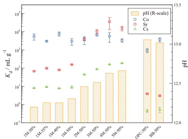
**Figure 4.** The pH of leachates (right (R) scale) and  $K_d$  values (left scale) of Co, Sr, and Cs for the geopolymer and cement samples.
