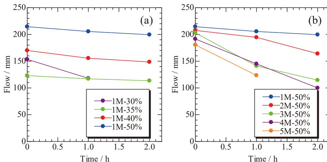
**Figure 1.** Temporal changes of the slump-flows for samples prepared using various amount of 1 M NaOH solution (a) and using constant amount of 1–5 M NaOH solution (b).
