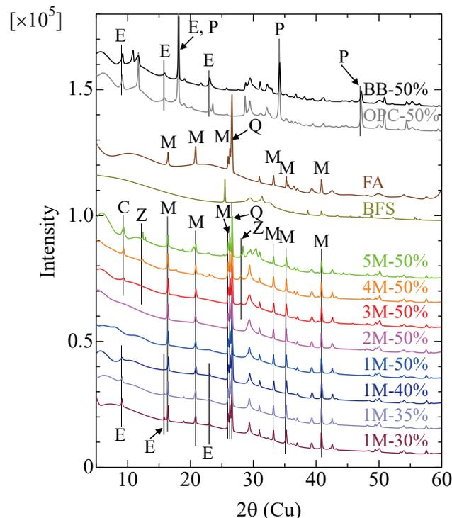
**Figure 5.** XRD spectra of the geopolymers, ingredients, and cements. C: chabazite, E: ettringite, M: mullite, P: portlandite, Q: quartz, Z: p-type zeolite.
