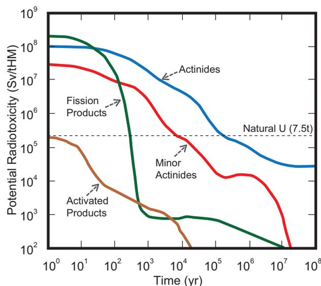
**Figure 1.** Potential radiotoxicity of radioactive nuclides generated in the fuel cycle of LWRs (normalized to 1 ton of new fuel) [1].
