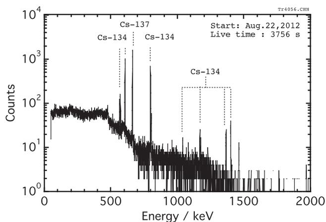
**Figure 2.** Gamma-ray spectrum of an SPM sampled at Kakinokizaka station (station code# 13-025) in Tokyo from 10:00 to 11:00 on March 15, 2011. The SPM sample was fixed at a distance of 4 mm from a Ge detector (GMX-30200S, ORTEC). A net area of 662 keV gamma-ray from  $^{137}\text{Cs}$  counted 6973, corresponding to 50 Bq.
