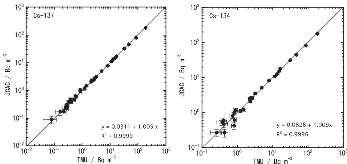
**Figure 3.** Comparison of  $^{134}\text{Cs}$  and  $^{137}\text{Cs}$  radioactivity concentrations (in  $\text{Bq m}^{-3}$ ) determined at TMU and JCAC for the same SPM samples. The lines in the graphs show 1:1 relationships between TMU and JCAC rather than regression lines of measured values.
