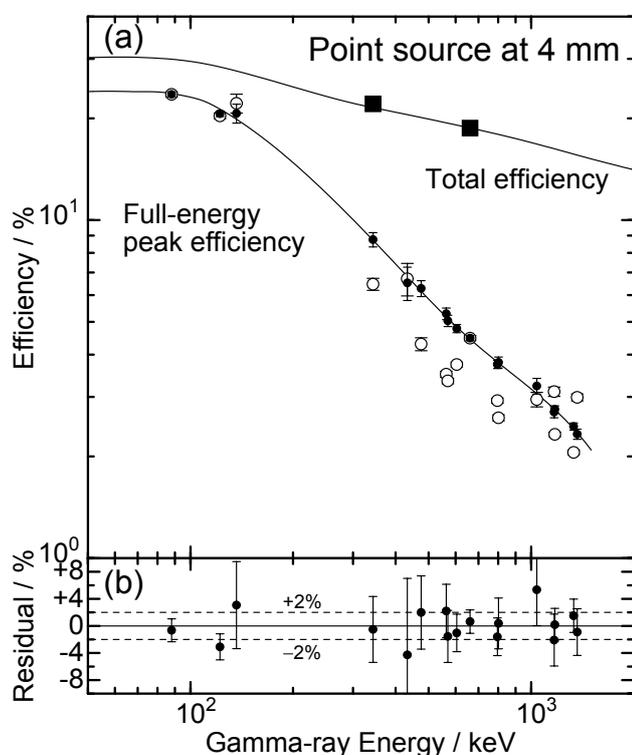
**Figure 7.** (a) Total and full-energy peak efficiencies for point sources placed at a source-to-detector distance of 4 mm. Open circles denote the efficiencies without cascade summing corrections, and closed circles denote the efficiencies with cascade summing corrections. A full-energy peak efficiency curve is obtained by fitting eq 1 to the corrected efficiencies. (b) Residuals of the corrected full-energy peak efficiency values to the fitted curve.
