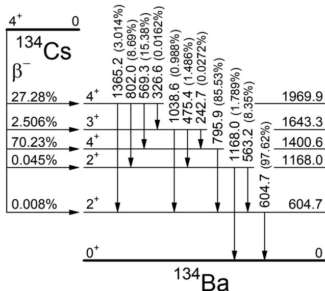
**Figure 2.** Decay scheme of  $^{134}\text{Cs}$ ,<sup>9</sup> with which we calculated the cascade summing corrections for the  $\gamma$  rays of  $^{134}\text{Cs}$ .
