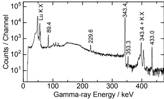
**Figure 6.** Gamma-ray spectrum observed with the  $^{175}\text{Hf}$  standard soil sample.
